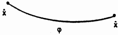
Fig. 3 Displacement of the x -axis under a rotation about the z -axis
